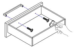
Attach handle in front of drawers, on the drilling hole position by using screwdriver to tighten bolts up.
